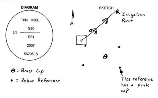
MONUMENT (S) AND ACCESSORIES SET (Procedures and Description) At the proportionate point I set a 1 1/2"x30 galvanized iron pipe with a 2 1/4" brass cap stamped as shown in the diagram above.
