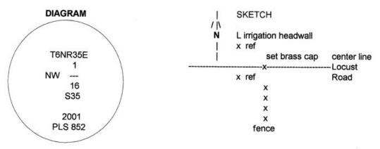
MONUMENT (S) AND ACCESSORIES SET (Procedures and Description) I set a 1 1/4" x 30" GIP with a 2 1/2" brass cap directly over Perry's found iron bar. The surface of the brass cap is at the top of the asphalt surface.
