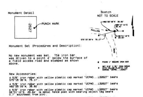
A  $5/8^\circ$  iron repar with yellow plastic cap marked "UCPWD...LSP627" bears N88 47 44 E, 38.40' (a 3' diameter iron pipe protruding 3.3' above ground with bearing object tag bears 0.9' northeast from pin).
