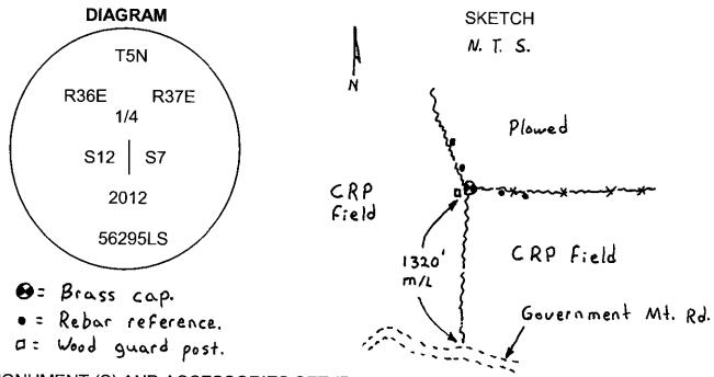
MONUMENT (S) AND ACCESSORIES SET (Procedures and Description) At the position of the stone I Set a 1 1/2" x 30" galvanized iron pipe with a 2 3/8" brass cap stamped as shown in the diagram above.
