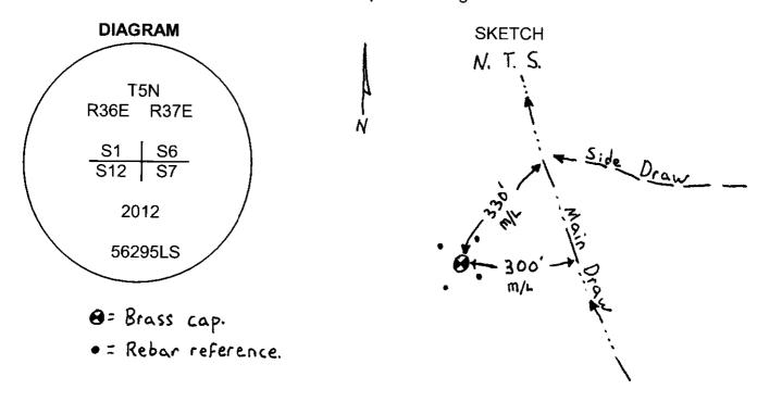
MONUMENT (S) AND ACCESSORIES SET (Procedures and Description) I set a 2 3/8" brass cap on a 1 1/2"x30" galvanized iron pipe with a brass cap stamped as shown in the diagram above 2 feet below the surface of the field at the proportionate point.
