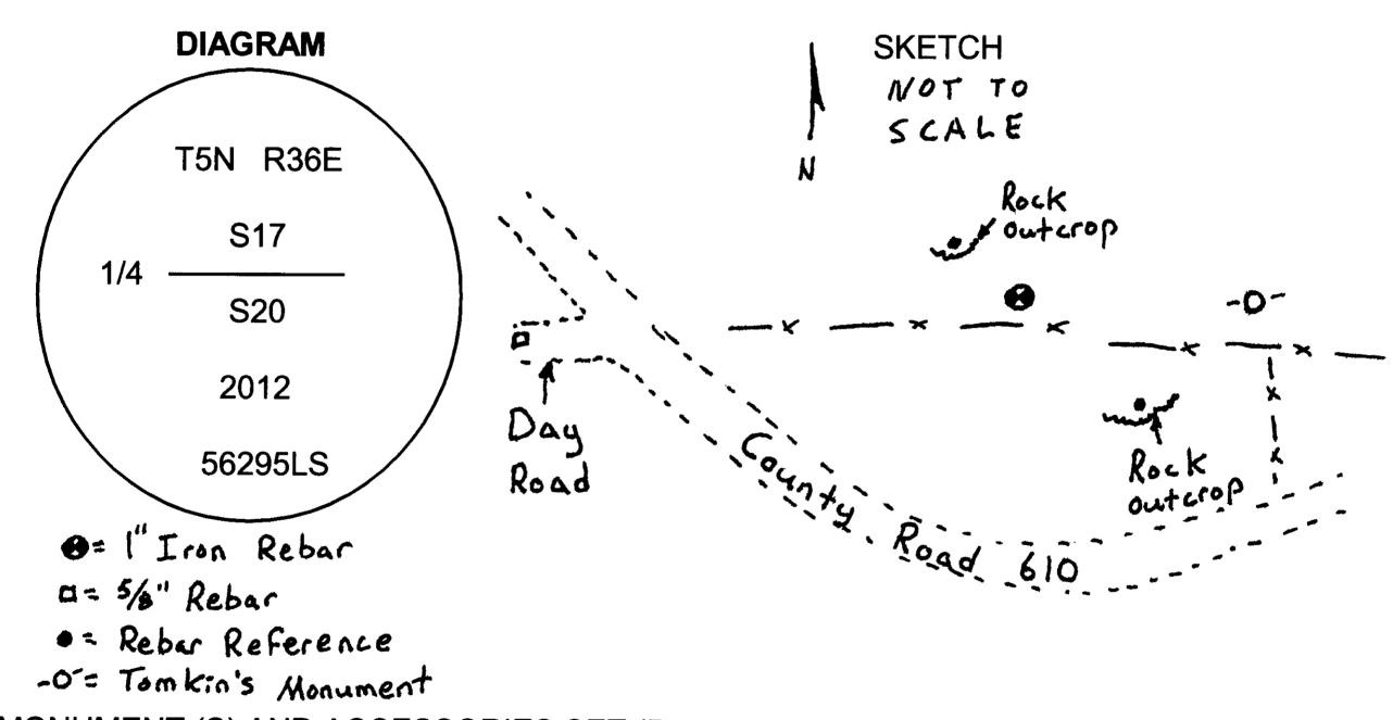
MONUMENT (S) AND ACCESSORIES SET (Procedures and Description) At the position of the 1/2" smooth iron rod, I drove a 1"x24" iron rebar 18" into the bedrock. I attached a 2" Aluminum cap stamped as shown in the diagram above and built a small
