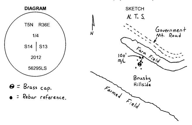
MONUMENT (S) AND ACCESSORIES SET (Procedures and Description) Set a 1 1/2" x 30" galvanized iron pipe with a 2 3/8" brass cap stamped as shown in the diagram above at the corner point
