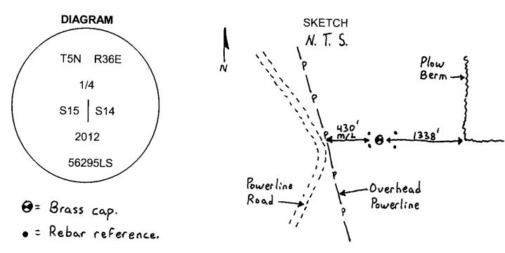
MONUMENT (S) AND ACCESSORIES SET (Procedures and Description) Set a 1 1/2" x 30" galvanized iron pipe with a 2 3/8" brass cap stamped as shown in the diagram above 2 feet below the surface of a plowed field.
