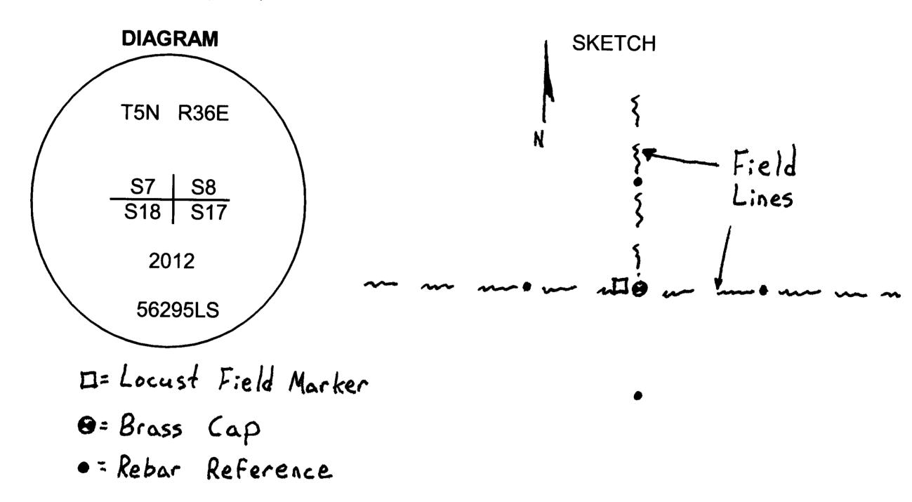
MONUMENT (S) AND ACCESSORIES SET (Procedures and Description) I set a 2 3/8" brass cap on a 1 1/2"x30" galvanized iron pipe with a brass cap stamped as shown in the diagram above at the position of the found stone.
