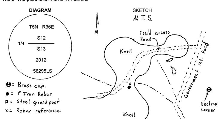
MONUMENT (S) AND ACCESSORIES SET (Procedures and Description) At the proportionate point I set a 1" x 24" iron rebar with a 2" aluminum cap stamped as shown in the diagram above 24" in the ground to bedrock.
