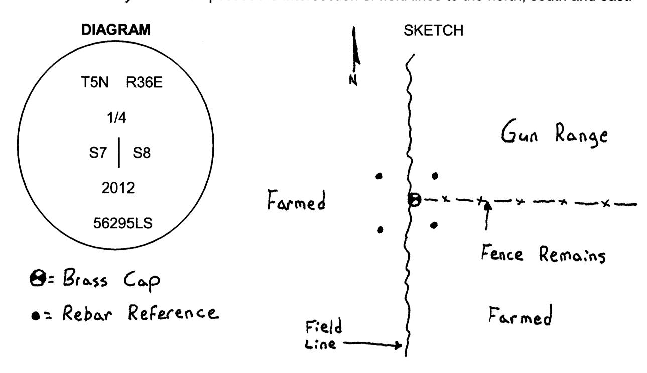
MONUMENT (S) AND ACCESSORIES SET (Procedures and Description) Set a 1 1/2" x 30" galvanized iron pipe with a 2 3/8" brass cap stamped as shown in the diagram above 2 feet below the surface at the position of the decayed wood.
