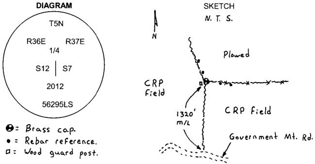
MONUMENT (S) AND ACCESSORIES SET (Procedures and Description) At the position of the stone I Set a 1 1/2"  $\times$  30" galvanized iron pipe with a 2 3/8" brass cap stamped as shown in the diagram above.
