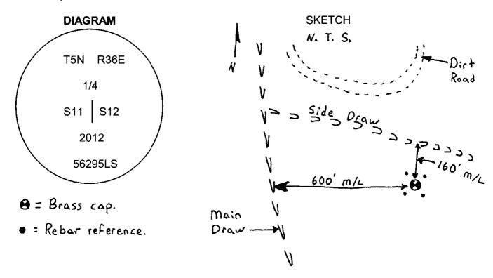
MONUMENT (S) AND ACCESSORIES SET (Procedures and Description) Set a 1 1/2" x 30" galvanized iron pipe with a 2 3/8" brass cap stamped as shown in the diagram above 2 feet below the surface of the plowed field at the proportionate point.
