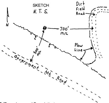
MONUMENT (S) AND ACCESSORIES SET (Procedures and Description) Set a 1 1/2" x 30" galvanized iron pipe with a 2 3/8" brass cap stamped as shown in the diagram above 2 feet below the surface of a plowed field at the proportionate point.
