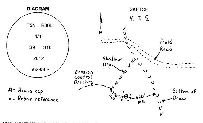
MONUMENT (S) AND ACCESSORIES SET (Procedures and Description) Set a 1 1/2" x 30" galvanized iron pipe with a 2 3/8" brass cap stamped as shown in the diagram above 2 feet below the surface of a plowed field at the proportionate point.
