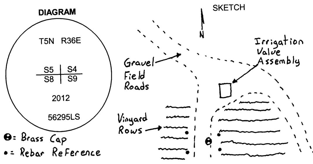
MONUMENT (S) AND ACCESSORIES SET (Procedures and Description) I set a 2 3/8" brass cap on a 1 1/2"x30" galvanized iron pipe with a brass cap stamped as shown in the diagram above at the intersection of the projected south and west lines of Section 4.
