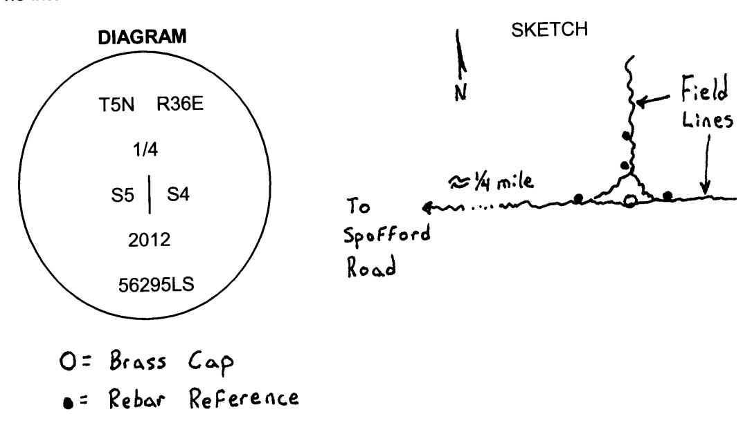
MONUMENT (S) AND ACCESSORIES SET (Procedures and Description) Set a 1 1/2" x 30" galvanized iron pipe with a 2 3/8" brass cap stamped as shown in the diagram above 2 feet below the surface of the plowed field at the intersection of the field lines.
