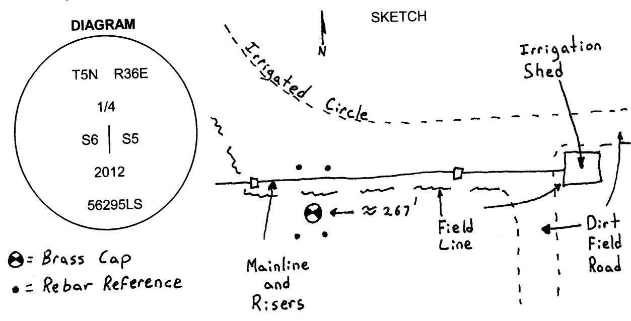
MONUMENT (S) AND ACCESSORIES SET (Procedures and Description) Set a 1 1/2" x 30" galvanized iron pipe with a 2 3/8" brass cap stamped as shown in the diagram above 2 feet below the surface of the plowed field at the proportioned point.
