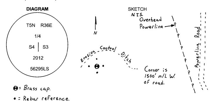
MONUMENT (S) AND ACCESSORIES SET (Procedures and Description) Set a 1 1/2" x 30" galvanized iron pipe with a 2 3/8" brass cap stamped as shown in the diagram above 2 feet below the surface of the plowed field at the proportioned point.
