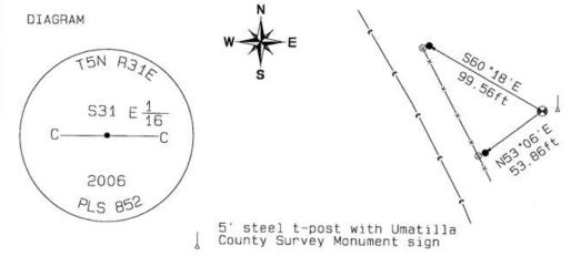
5/8"dia. x 30" long Iron Rebar with a 1.3"dia. Set 2"dia. Aluminum cap on a 5/8" x 30" long Iron Rebar. ⊗ Wood fence post Red plastic cap.
