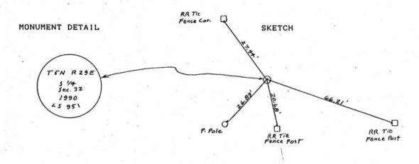
MONUMENT SET (PROCEDURES AND DESCRIPTION) Set 2 1/2" BC stamped as above over a 1/2" rebar which is over the 1" bolt. Set at the surface of paved road in concrete.
