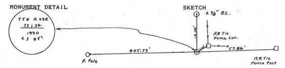
MONUMENT SET (PROCEDURES AND DESCRIPTION) Set a 2 1/2" Brass cap stamped as above in concrete in top of existing 1 1/4" iron pipe.
