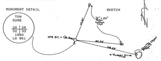
MONUMENT SET (PROCEDURES AND DESCRIPTION) By retracing Eriksen's 1917 survey | set a 1"x 30" | Iron pipe with 2 3/8" Brass Cap, stamped as above, in a swamp. Placed a 16" piece of 24" P.V.C. and filled with sand to level of top Brass Cap. See Umatilla County 1989 Area One Survey.
