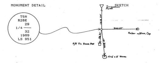
MONUMENT SET (PROCEDURES AND DESCRIPTION) By single proportion (See County Survey Area One 1989), I set a 2 1/2" Brass Cap Disc, stamped as above, in a 6"x10" concrete cylinder with a 3/4" x 29" Iron rod imbedded. Disc is 20" below surface of cultivated field.
