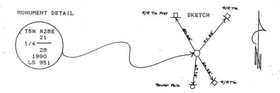
MONUMENT SET (PROCEDURES AND DESCRIPTION) Set a 1"x30" Galv. pipe with a 2 3/8" Brass Cap, stamped as shown. Found pipe was undisturbed. New Brass Cap is flush with asphalt road surface and a concrete patch was poured around cap.
