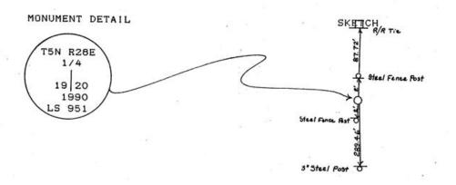
MONUMENT SET (PROCEDURES AND DESCRIPTION) Set by single proportion a 1"x30" Iron pipe with a 2 3/8" Brass Cap 0.20 ft. above surface of ground and stamped as shown.
