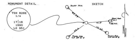
MONUMENT SET (PROCEDURES AND DESCRIPTION) Over found 1 1/2" l. Pipe, set a 2 1/2" Brass Cap in conc. at 0.3 ft. below ground level, stamped as shown.
