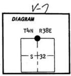
A Pine 9 inches diameter bears N15°E, 13 1ks dist marked  $\frac{1}{4}$  S29 BT A Pine 12 inches diameter bears South 22 1ks dist marked  $\frac{1}{4}$  S32 BT
