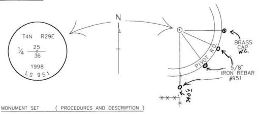
BY SINGLE PROPORTION I SET A 1" X 30" IRON PIPE WITH A 2 3/8" BRASS CAP STAMPED AS ABOVE, 20" BELOW THE SURFACE OF A CULTIVATED FIELD.
