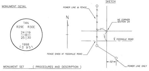
BY SINGLE PROPORTION, I SET A 1" X 30" IRON PIPE WITH A 2 3/8" BRASS CAP STAMPED AS ABOVE. 4" BELOW THE SURFACE OF A DIRT ROAD,
