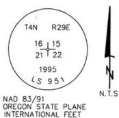
6 FOOT N 3\*35'59' € 1/2" x 24" IRON ROD 0.96" WITH ALUM. CAP 2 89.06.30. A N 89.05.18. € 5/8' × 30' IRON ROD VO-WITH YELLOW PLASTIC CAP. 9.97 9.97 SECTION CORNER MKD "#951" 1 1/4" x 33" IRON ROD WITH AN ALUM. CAP MKD '#951'
