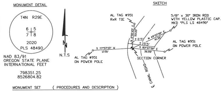
PLACED A 2" ALUMINUM CAP ON EXISTING 5/8" IRON ROD, STAMPED AS ABOVE.
