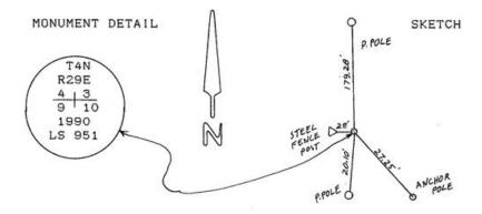
MONUMENT SET (PROCEDURES AND DESCRIPTION) I poured 8" cylinder of concrete 8" deep over Iron pipe and placed 3" Brass Disc over it.
