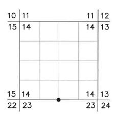
**ORIGINAL DESCRIPTION:** Set a basalt stone  $15 \times 10 \times 8$  ins 10 ins in ground on SE slope for 1/4 sec. cor marked 1/4 on N. face
