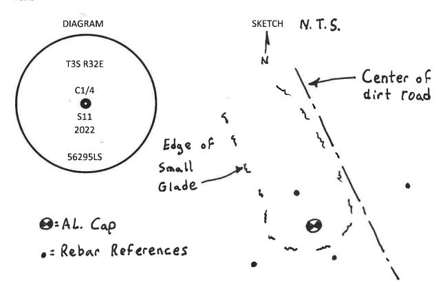
MONUMENT(S) AND ACCESSORIES SET (Procedures and Description) At the point calculated per the manual of instructions I set a 2 3/8" aluminum cap on a 2 3/8" x 30" aluminum pipe 26 inches in the ground to bedrock. The cap was stamped as shown in the diagram above.
