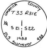
B.T.'s: A 11" diameter Douglas Fir Bears South  $79^{\circ}$  East a distance of 39.73 feet scribed,  $\frac{1}{8}$  S 22 BT.
