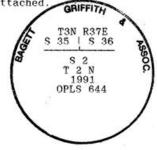
I used a steel tape and magnetic compass in the establishment of new accessories. I used 20° East magnetic declination and the distances are to a 50d spike driven in the right side of the root crown. I attached a brass washer marked OPLS 644 to the BT blaze.
