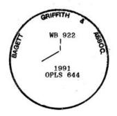
I used a steel tape and magnetic compass in the establishment of new accessories. I used  $20\,^\circ$  East magnetic declination.
