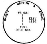
I used a steel tape and magnetic compass in the establishment of new accessories. I used 20° East magnetic declination and the distances are to a 50d spike driven in the right side of the root crown. I attached a brass washer marked OPLS 644 to the BT blaze.
