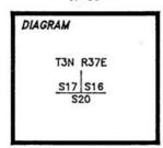
2002, David A. Schlaich, Registered Land Surveyor No. 2308, found on the northwest slope of a spur ridge a basalt stone 17" X 12" X 7", projecting 4" out of the ground, with 4 notches on the East edge and 3 notches on the southerly end of the top edge, from which:
