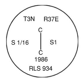
I used a steel tape and magnetic compass in the establishment of the new accessories. I used 13° East declination, the distances are to a 60d spike driven into the right side of the root crown of the bearing trees. A brass washer marked OPLS 83571 is attached to the BT blaze of the new bearing trees.
