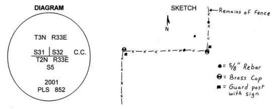
MONUMENT (S) AND ACCESSORIES SET (Procedures and Description) Set a 2 1/2" brass cap on a 1 1/4" x 30 galvanized iron pipe stamped as shown in the diagram above at the position indicated by the old fence corner. Set a wooden post with a county monument sign attached along side.
