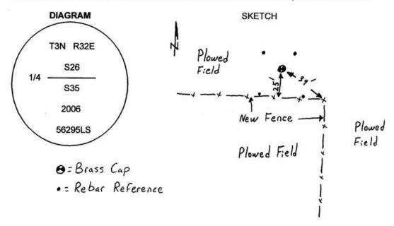
MONUMENT (S) AND ACCESSORIES SET (Procedures and Description) I set a 1 1/4" x 30" galvanized iron pipe with a 2 3/8" brass cap stamped as shown in the diagram above at the proportionate point. The top of the monument is approximately 2' below the surface of the ground.
