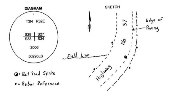
MONUMENT (S) AND ACCESSORIES SET (Procedures and Description) At the intersection of the State Highway centerline from the north and the field lines to the west I set a railroad spike in the asphalt stamped with an "+" and the section numbers.
