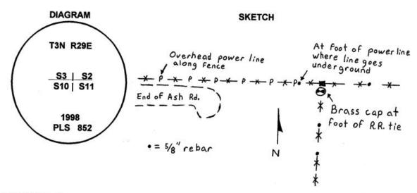
MONUMENT (S) AND ACCESSORIES SET (Procedures and Description) At the intersection of a fence with fences running East, West, and South we set a 2 1/4 inch brass cap on a 1 1/8" x 24" galvanized iron pipe flush with the surface of the ground.
