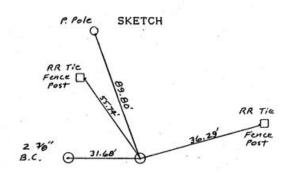
MONUMENT SET (PROCEDURES AND DESCRIPTION) By retracing Goulds 1940 Survey I set a 1"x 30" I Pipe with a 2 3/8" BC, stamped as above, .4 foot below the surface of a graveled road. See Co. Survey # 90-52-A
