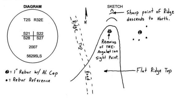
MONUMENT (S) AND ACCESSORIES SET (Procedures and Description) At the position of the original stone I set a 1" x 24" iron rebar with a 2" aluminum cap stamped as shown in the diagram above. I merely moved the original stone over and left the mound undisturbed when setting the rebar. I did not add any new stones to the mound.
