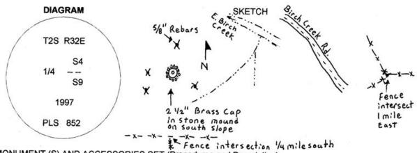
MONUMENT (S) AND ACCESSORIES SET (Procedures and Description) Set a 1 1/4" x 30" Galvanized Iron Pipe with a 2 1/2" brass cap stamped as shown in the diagram above at the position of the stone. Raised a mound of stone around the monument.
