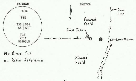
MONUMENT (S) AND ACCESSORIES SET (Procedures and Description) At the corner point determined by the fences I set a 2 3/8" brass cap on a 1 1/2"x30" galvanized iron pipe 36" in the ground.
