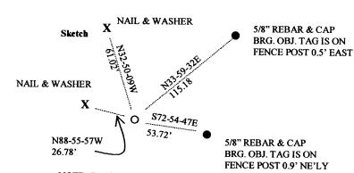
NOTE: Bearings are grid rotated 1-14-39 Clockwise to true
